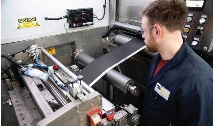
ALL AMPED UP: Bye Aerospace's eFlyer 2 [top] is designed to train pilots. Bye is working with Oxis Energy on a lithium-sulfur battery that promises to increase the plane's range. Here a reel of positive electrode, made of sulfur, is being coated onto a current collector [bottom].
